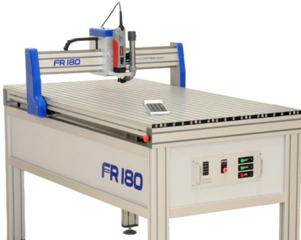
Figura C.1: Fresadora Alarsis FR180 (Alarsis).
